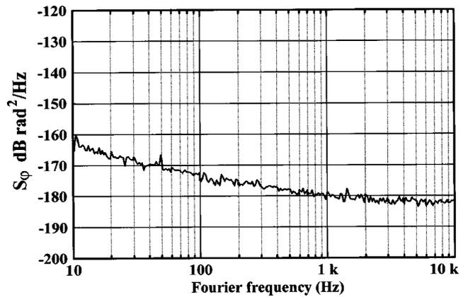
FIG. 5. Instrument phase noise  $S_{\varphi_0}(f)$  of the microwave NMS prototype measured at  $\nu_c=9.13$  GHz and DUT power  $P_o=14$  dBm.
