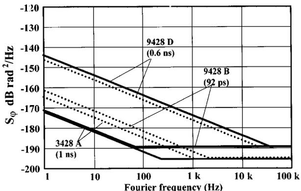
FIG. 8. Phase and amplitude noise of some microwave phase shifters measured at  $\nu_c=100$  MHz. Solid line: phase noise  $S_{\varphi}(f)$ ; dotted line: amplitude noise  $S_a(f)$ .
