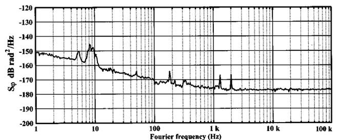
FIG. 6. Instrument phase noise  $S_{\varphi_0}(f)$  of the VHF NMS prototype measured at  $\nu_c=100$  MHz and DUT power  $P_o=9$  dBm.
