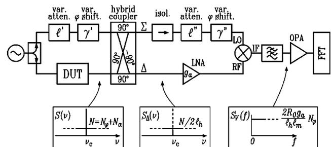
FIG. 2. Scheme of the interferometric phase noise measurement system.
