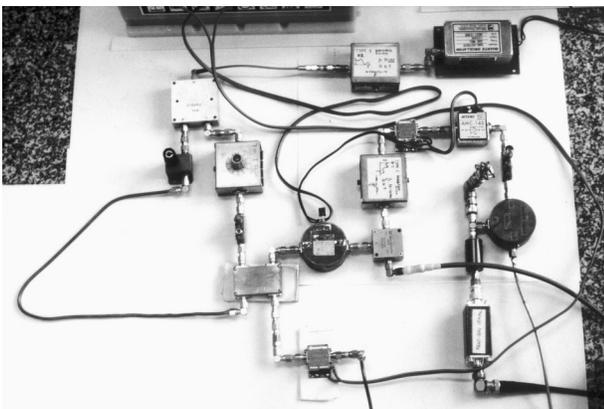
FIG. 4. VHF prototype of interferometric noise measurement system.
