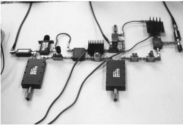
FIG. 3. Microwave prototype of interferometric noise measurement system.
