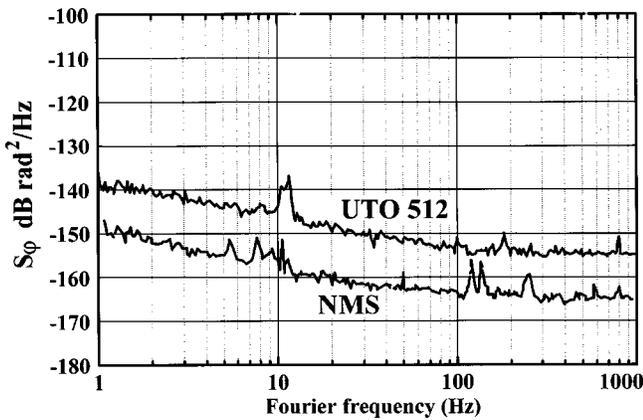
FIG. 7. Phase noise  $S_{\varphi}(f)$  of a UTO 512 amplifier measured at  $\nu_c=100$  MHz in weak signal conditions. The actual output power is  $P_o=0$  dBm, while the 1 dB compression power is  $P_m=+8$  dBm. The instrument noise of the NMS is also reported.
