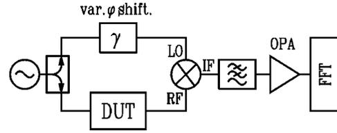
FIG. 1. Scheme of the traditional phase noise measurement system based on a saturated mixer.
