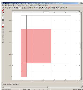
Fig. 2: Geometry used for F.E. simulation.
