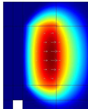
Fig. 3:  $WGH_{15,0,0}$  magnetic field configuration simulated by F.E..
