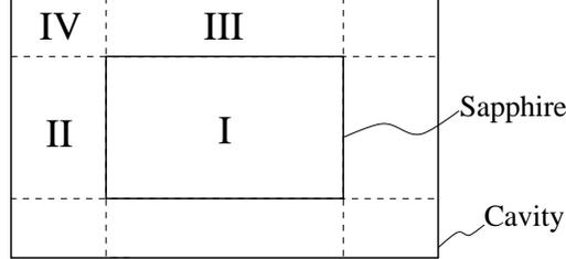
Fig. 5: *Sapphire Resonator Modeling for Mode Matching.*
