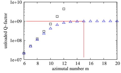
Fig. 6: *Sapphire resonator frequencies for  $WGH_{m,0,0}$  modes at 4 K.* Fig. 7:  $\triangle$ : *Q-factor for  $WGH_{m,0,0}$  modes;  $\square$ : contribution of metallic losses at 4 K*
