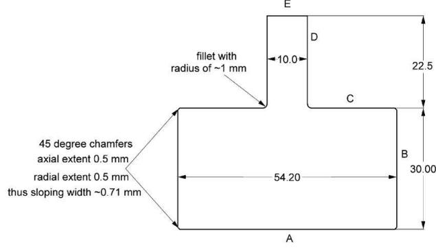
Fig. 4: Sapphire resonator geometry
